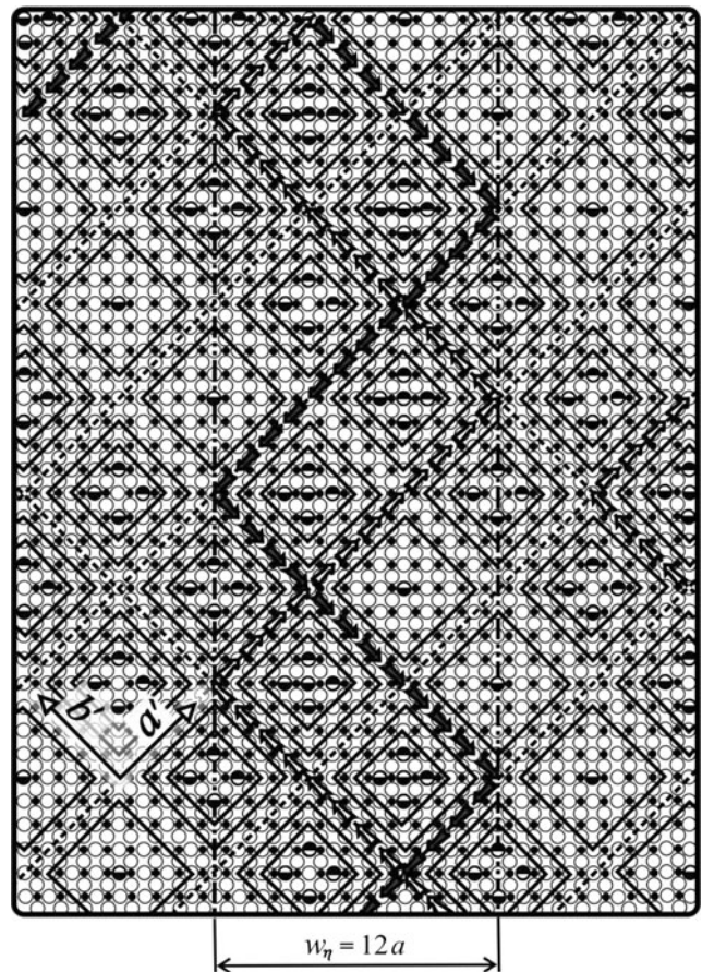
Fig. 2 Sketch of simulated hole trajectories and appropriate distribution of oxygen interstitials in a fragment of \text{La}_2\text{CuO}_{4+\delta} with \delta \approx 1/8 . The localized hole orbitals in the \text{CuO}_2 layer are denoted by solid lines (rhombs) , while the zigzagging trajectories belonging to twelfth-rank BS with T_{c\eta}^*(\delta) = 40 K are depicted by arrows . Projections of oxygen interstitials from the adjacent \text{La}_2\text{O}_{2+\delta} layers placed above and below the given fragment of \text{CuO}_2 are marked by symbols \ominus and \omin� , respectively. The dashed lines denote the 12a' \times 4b' superstructural cells
